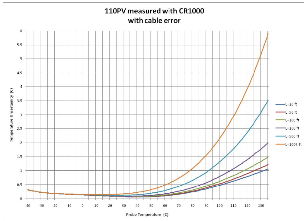
FIGURE 2-5. 110PV measured with a CR1000 showing effects of cable length
